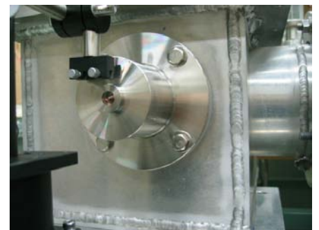
Fig.1 Winston cone for the illumination probe.
